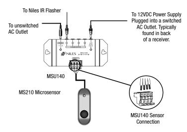
Figure 2: MSU140 Installation
